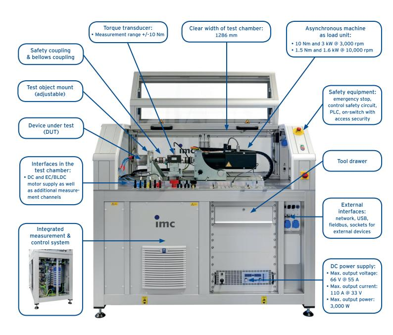
Test stand dimensions with hood open: 1650 x 800 x 2000 mm (W x D x H)
