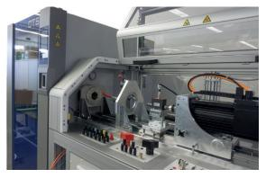
EC/DC motor test stand with climate chamber
