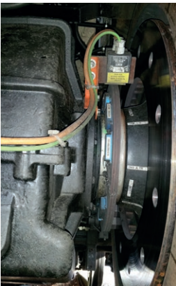
Force measurement on railway wheel set
