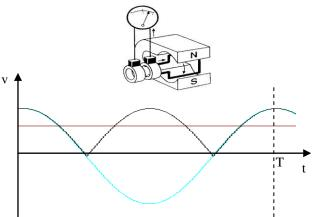
To imagine a three-phase generator we add two independent wire windings. Now we have 3 sine wave voltages which are spaced about 120° out of phase. After three-way rectification with six diodes the result is an alternating DC voltage with 6 pulses per revolution (black line) and an increased average voltage against the generator with one winding.
