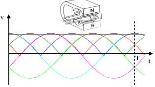
In practice generators for automobiles have more than two poles. In most cases here we find 12 poles (6 pole pairs) and sometimes also 16 poles (8 pole pairs). For the first one we get from every phase 6 cycles per revolution and after rectification an alternating DC voltage with 36 pulses.
