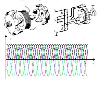
The board net voltage ripple frequency can simply calculated by multiplying the alternator RPM with the number of poles (e.g. 12\*2=24) and the number of phases (3). 12\*2\*3=72
