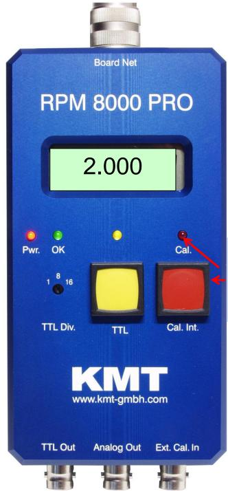
When a constant speed of 2000 rev/min is registered by the vehicle tachometer, press the Cal. Int. button until the red LED stops flashing, and remains constantly illuminated.
