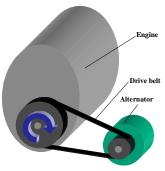
By connecting to an automotive cigarette lighter socket the measurement unit RPM-8000 PRO senses the small AC ripple of the vehicle board net DC supply voltage and generates on its outputs both a TTL digital pulse train and an analog voltage signal. These signals are "per design" linear to the alternator RPM and by the linear drive belt relationship also to the engine RPM. The scaling factor can determined by the relation between the effective diameters of the engine and the alternator pulleys.
