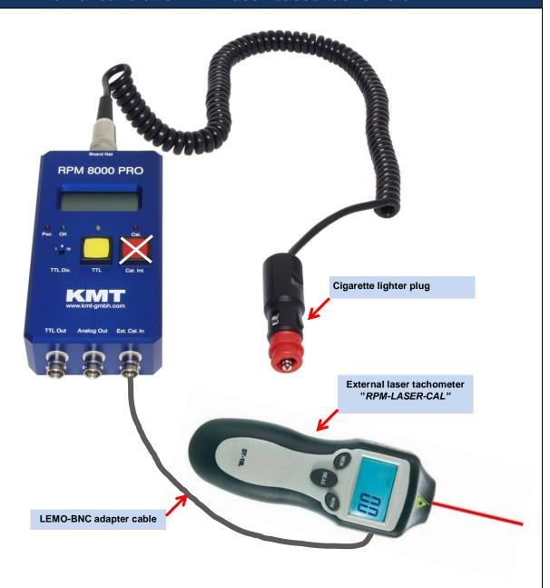
Attach a reflector tag (approximately 10 mm long) to the calibration shaft (crankshaft).
