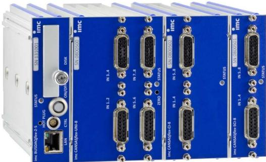
imc CANSASflex modules connected (Click-mechanism)
